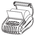
b. Correctly install the paper roll.
